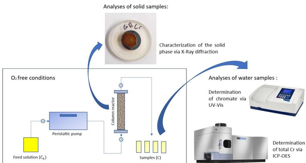
Fig.2 Schematic working set-up used for the reactivity experiments (free oxygen conditions): the collected water samples were analysed spectrophotometrically (determination of the Cr(VI) content) and via ICP-OES
