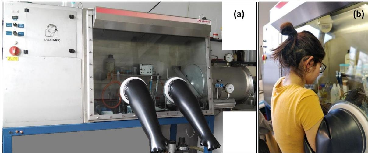
Fig.1 (a) The glovebox for the experiments in Oxygen-free atmosphere, (b) Flavia during one of her experiments under anoxic conditions.
