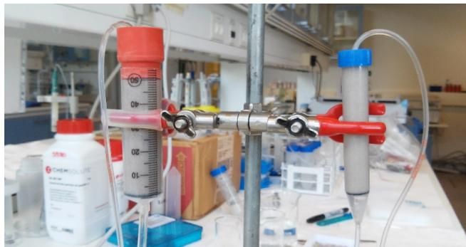
*Figure 1 Water-saturated columns used for the preliminary and tracer tests (University of Copenhagen).*
