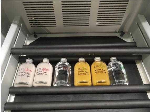
**Figure 1** (above) Batches of the long-term experiment of siderite dissolution in the presence of Pb (left) and Cu (centre) under exception of oxygen on a rotary shaker in the geochemistry laboratory of Section 4.4, GFZ.
