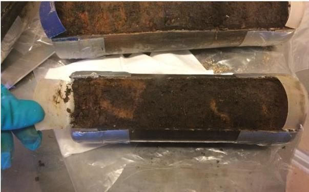
This photo shows one of the sediment cores, which were taken in Iceland and then analysed during the secondment at the University of Copenhagen. The whole work was done under Oxygen-free atmosphere in a glove box.
